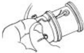
3.5 Untie and remove the ground strap (12)
